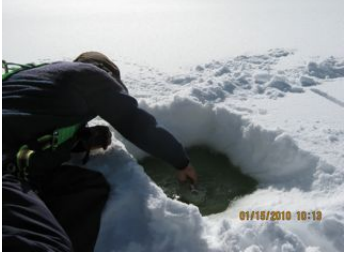
Above and to left is pictured the access hole utilized to collect samples. This is at the withdrawal sump (note location relative to orange float) and water depth was measured to be approximately 5'7". With outfall hose four feet below float, it is likely that water flowing through outfall to sample tap is affected by proximity to reservoir floor.
