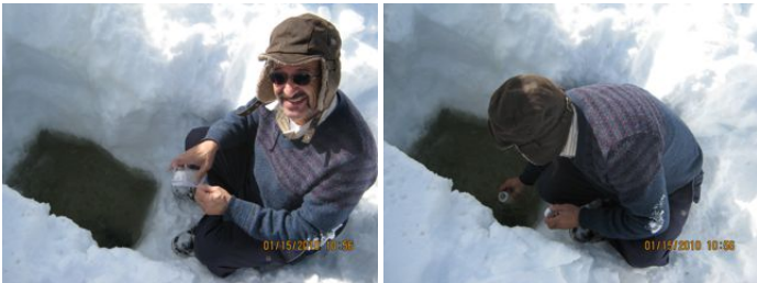
Above and to left is pictured the access hole utilized to collect samples. This is at the withdrawal sump (note location relative to orange float) and water depth was measured to be approximately 5'7". With outfall hose four feet below float, it is likely that water flowing through outfall to sample tap is affected by proximity to reservoir floor.
