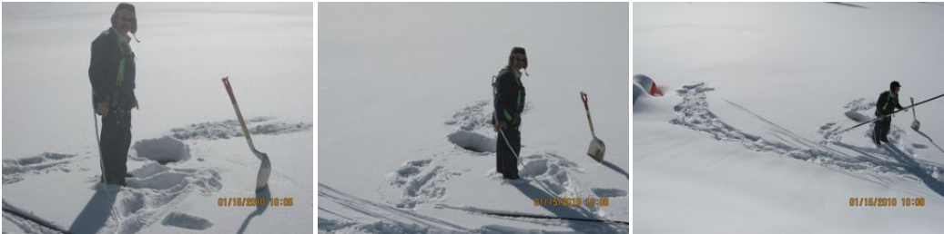
Above and to left is pictured the access hole utilized to collect samples. This is at the withdrawal sump (note location relative to orange float) and water depth was measured to be approximately 5'7". With outfall hose four feet below float, it is likely that water flowing through outfall to sample tap is affected by proximity to reservoir floor.
